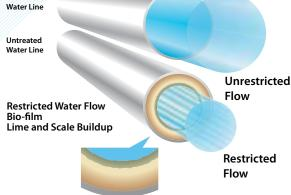
An untreated water line contains biofilm, causing potential health risks and water flow restriction
